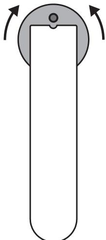
If necessary, rotate the spout escutcheon so that the hole for the pull rod aligns with the notch on the back of the spout.
