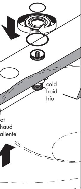
For proper operation of the faucet, the hot valve must be on the left, and the cold valve must be on the right.
