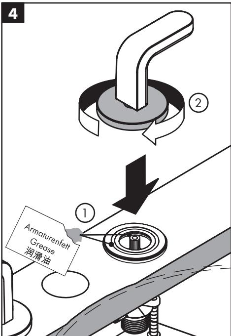
Lightly lubricate the valve stems and the threads on the handle mounting plates using white plumbers' grease.
