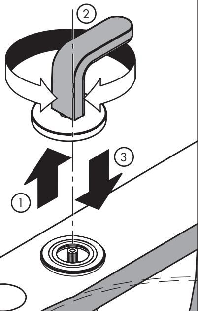
If necessary, remove, rotate, and reinstall the handle.
