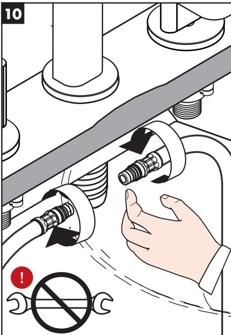
Screw the connecting hoses into the spout tee by hand.
