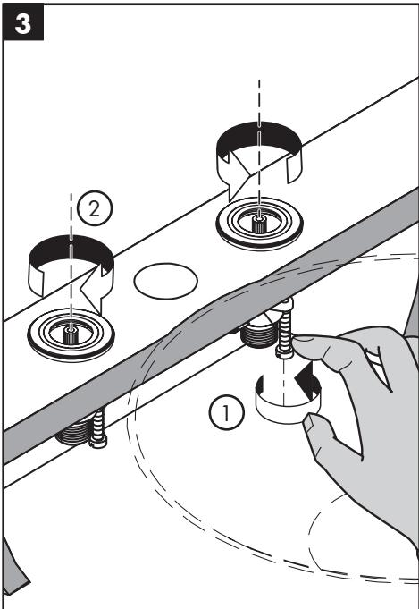
Tighten the tensioning screws by hand.
