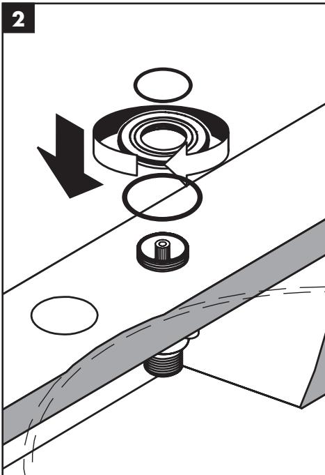
Install the mounting nuts on the valves.
