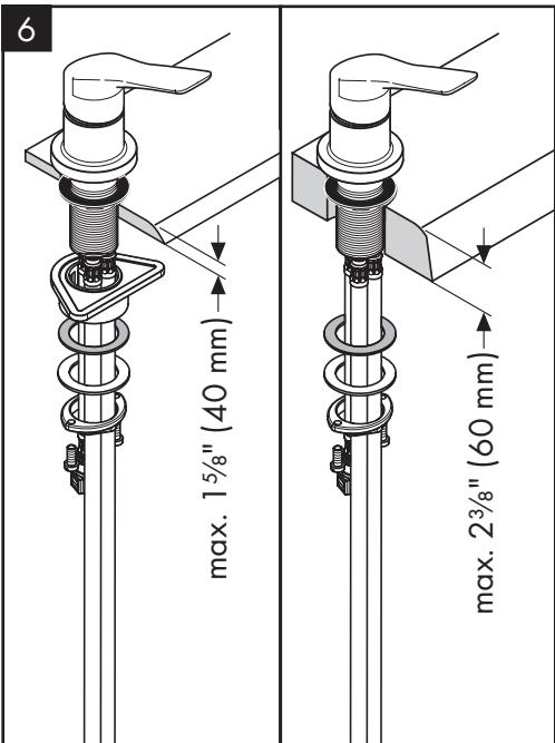
Place the valve and sealing ring on the mounting surface.
