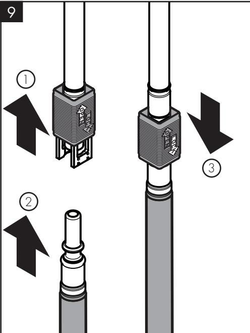
Open the quick connect by pushing it upwards.
