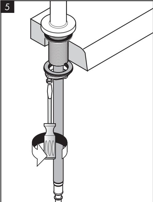
Tighten the mounting nut.
