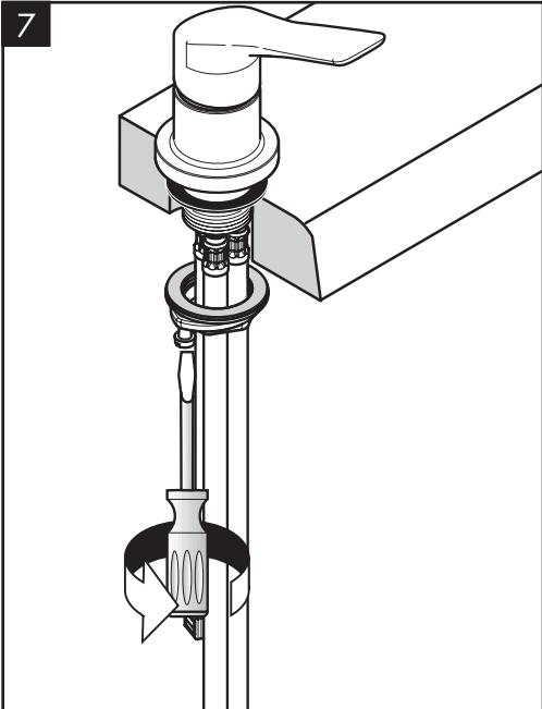
Tighten the mounting nut.
