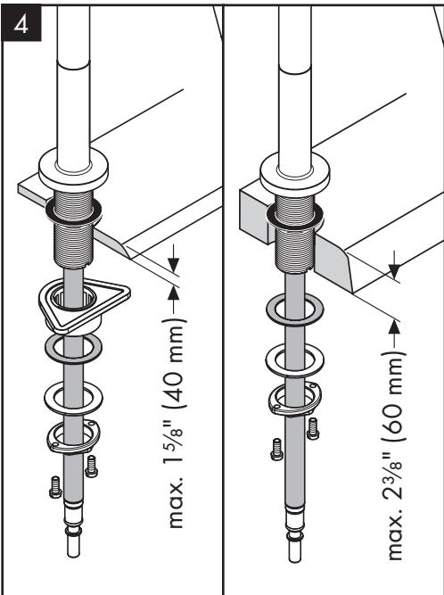
Place the spout and sealing ring on the mounting surface.
